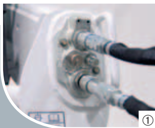
The hydraulic quick couplers ① are fixed directly to the front plate of the lifting arm, providing a solid mounting. The quick coupler hoses are run inside the loader arms for better protection.
